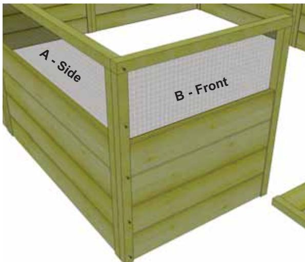
**8.** Align and attach remaining **Side Panels (Part A)** and **Front Panel (Part B)** as per **Steps 2, 3 & 4**. Attach with **5 - 2 1/2" Screws** per panel.
