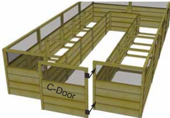
**21.** Attach Door to front wall framing with **3 - 3/4" Black Headed Screws** per hinge. Pre-drill shallow hole first to prevent wood from splitting.
