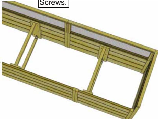
**18.** Complete remaining short **Bed Rib Frames (7)** as per **Step 17**.
